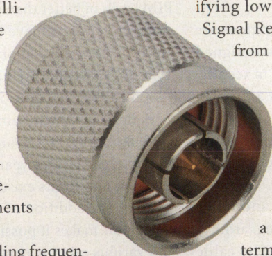
2. The Type-N connector, developed around the time of World War II, provides reliable performance from dc to 11 GHz. (Photo courtesy of Amphenol RF, www.amphenolrf.com )
